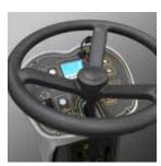
Control panel with digital controls and display. Digital display: with hour meter, battery charge level indicator, empty water tank level indicator and forward/reverse traction indicator, speed control adjustment, horn, suction motor
