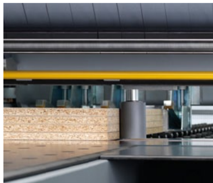
Double performance pressure unit – uncompromisingly precise positioning against the mitre fence.
