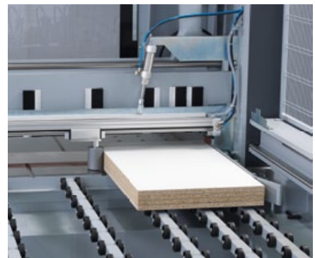
Roller tracks on the rear support table for smooth panel handling to the cutting line.
