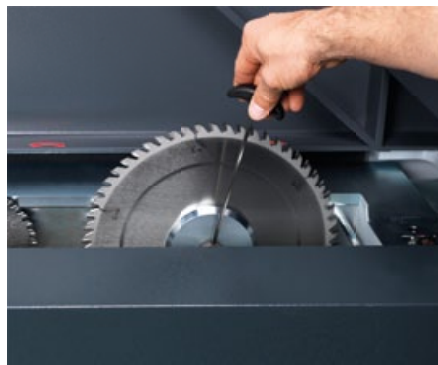
ProLock® Easyfix saw blade quick-change system guarantees shortest setup times.
